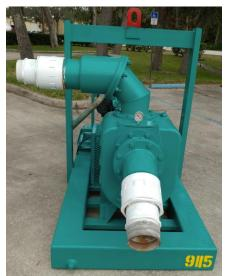
Completely refurbished by the OEM Flow rates to 2400 GPM, 120' head Deutz 6cyl. T6L912 (Torpedo) air cooled engine 8" ITT Marlow Self-Priming Trash pump 3" solids capacity; Frame mounted
