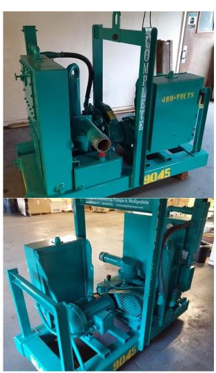
Completely refurbished by OEM capacity to 700 GPM, heads to 40'TDH Complete CP4 wet end, C3 vacuum pump 20Hp World Wide Electric 230/460V TEFC motor
